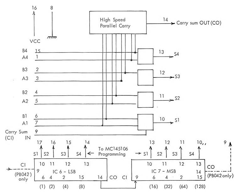
Al to A4 are determined by setting of Channel Selector (binary 15 to 59); Bl to B4 are binary numbers which are generated by the setting of the BAND Switch and when added to the Channel Selector binary numbers give logic"1" or "0" outputs at Sl to S4, which are in turn applied to the binary programming of the PLL pins.
