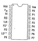
\*1 = 10 KHz steps, 0 = 5 KHz stsps \*1 = Locked, 0 = Unlocked
